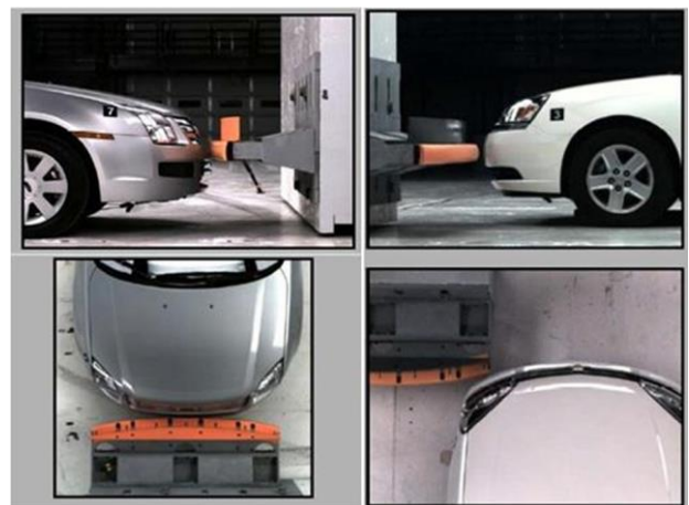
Fig. 5. Snaps during frontal and corner impact test
